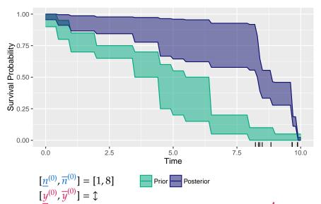
$$R_{\text{sys}}(t \mid \bigcup_{k=1}^{K} \{n_{k,t}^{(0)}, y_{k,t}^{(0)}, t^{k}\}) = P(T_{\text{sys}} > t \mid \cdots)$$
